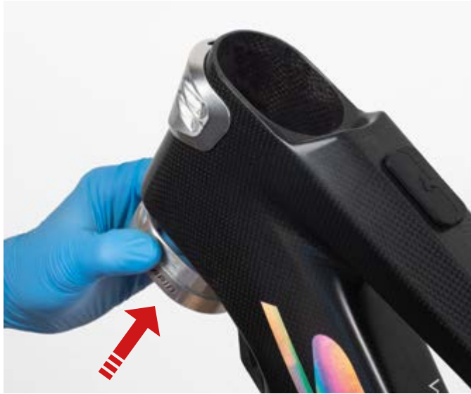
1. Insert the lower ISA headset adapter.
