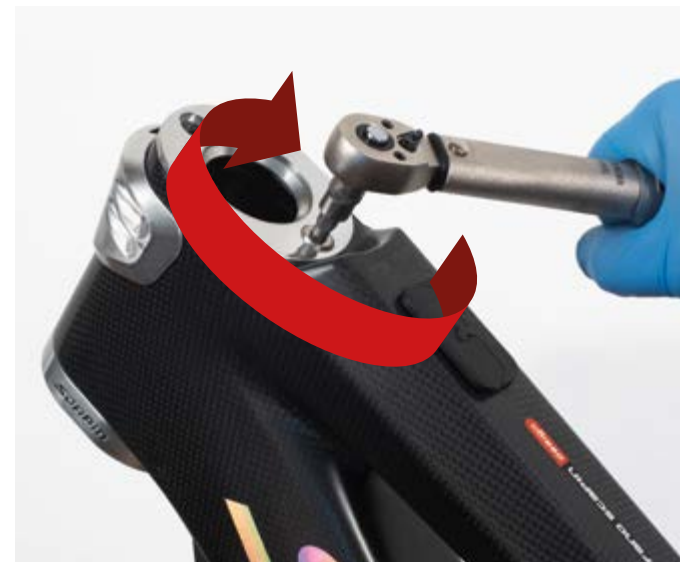
6. Tighten the screws with the torque wrench to a torque of 4 Nm.
