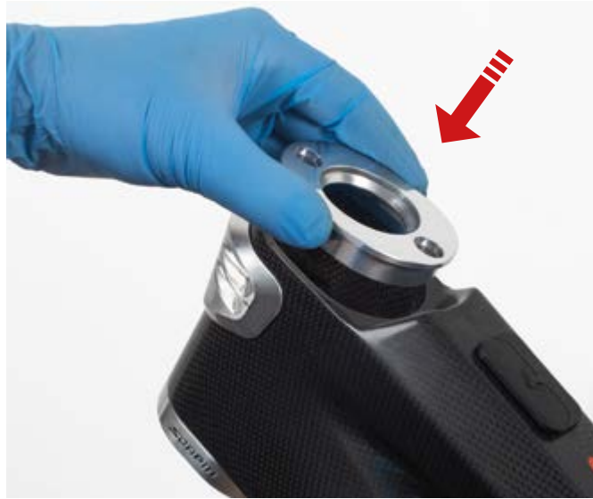
2. Insert the upper ISA headset adapter.
