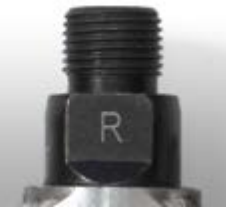
Right pedal - screw clockwise.
