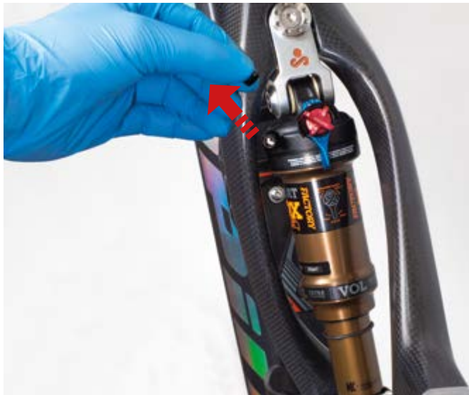
1. Unscrew the air filler valve cap.
