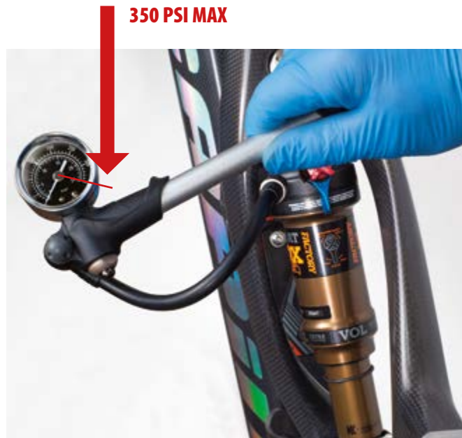
2. Insert the high pressure pump and supply air up to the desired pressure. Refer to the table in the manufacturer's manual for the correct pressure value based on your weight. Finally, unscrew the pump fitting and screw the valve cap back on.
