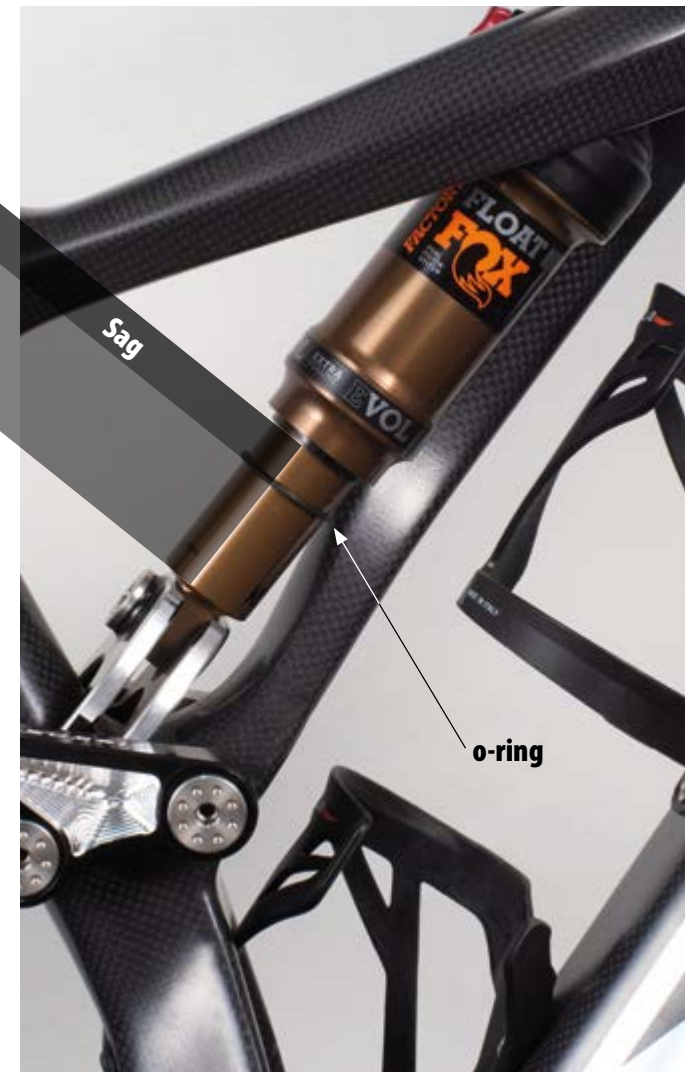
3. Adjust the sag according to your weight and riding style.
