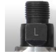
Left pedal - screw counter-clockwise.
